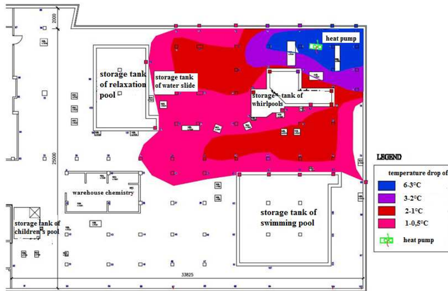
Figure 4. The map of the cooling of aqua park engine room - heat pump (air/water) is located under the relaxation pool
